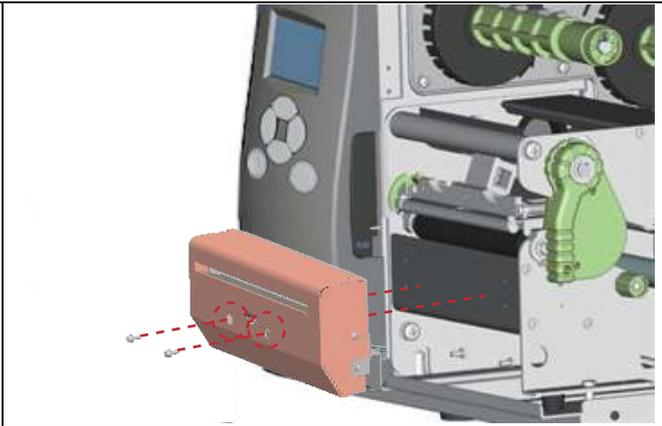
4. Connect the cutter cable connector to the cutter jack on the printer.
