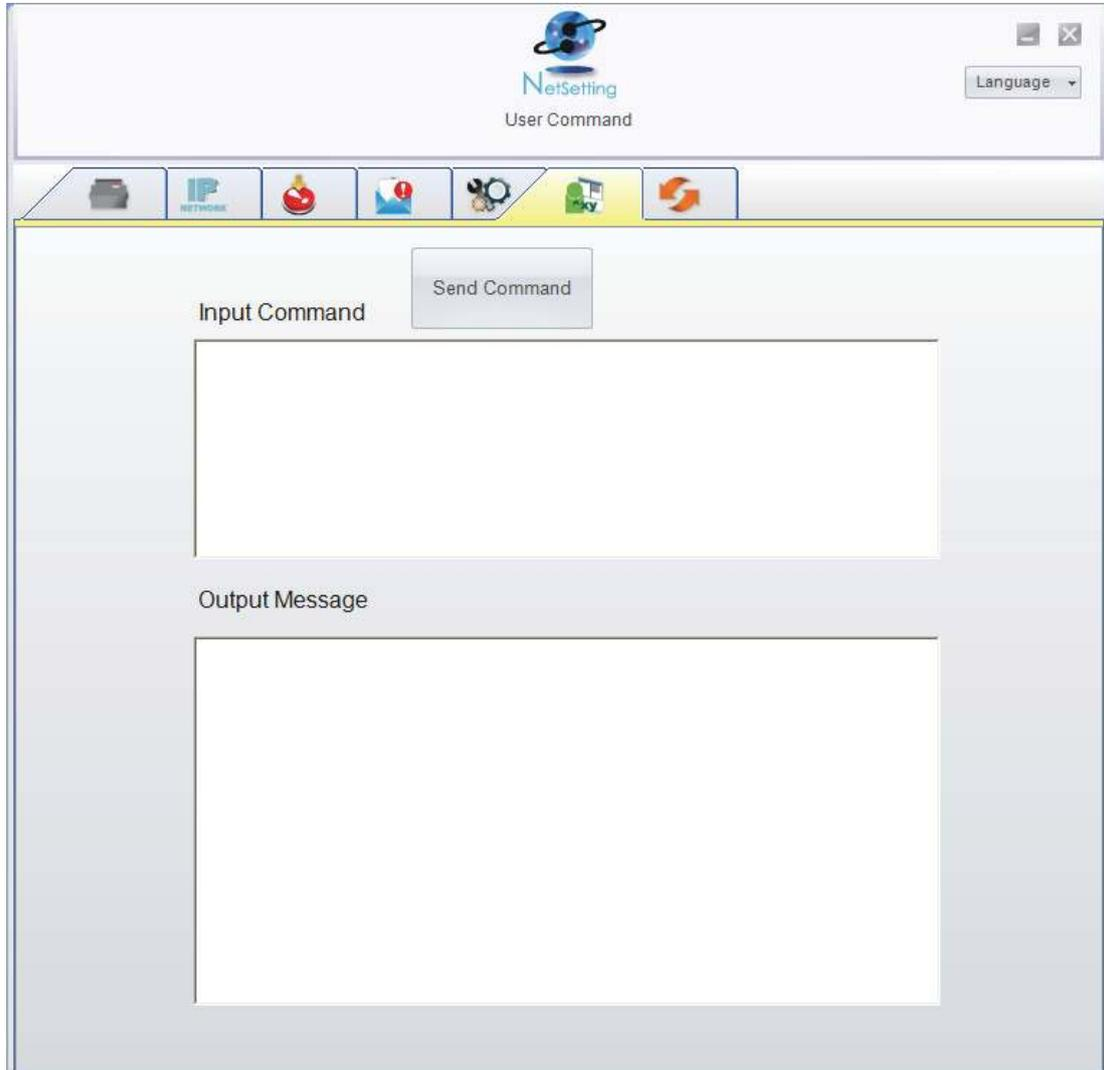
You can press "Send Command" button to send printer commands via Ethernet port and control the printer remotely.
