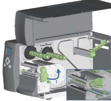
A 3D cutaway illustration of the printer's interior. A blue arrow points to a lever being lifted upwards. An inset image shows a close-up of the lever being moved.                                      |
