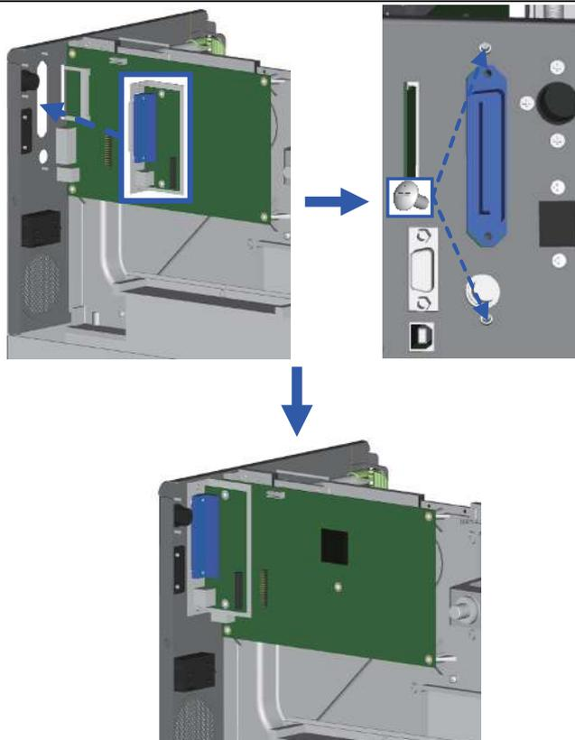
5. Connect the 30-pin connection cable to the motherboard.
