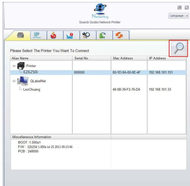
Click the magnifier icon to search the Godex printers which are connected via Ethernet port in your network environment. Once a connected Godex printer is detected, it will be listed on the start page.
