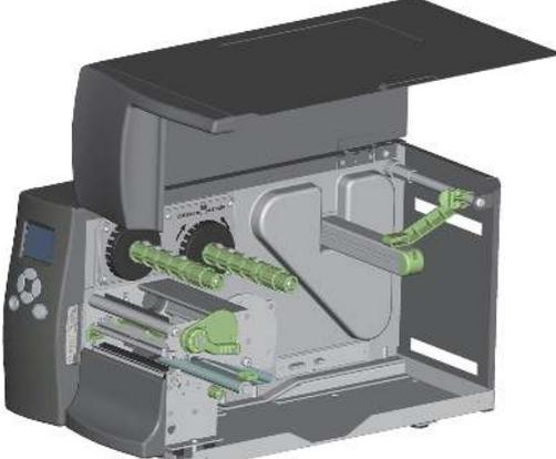
A 3D cutaway illustration of a printer with its top cover open, showing the internal print head assembly. The print head module is highlighted in green.                                                  |
