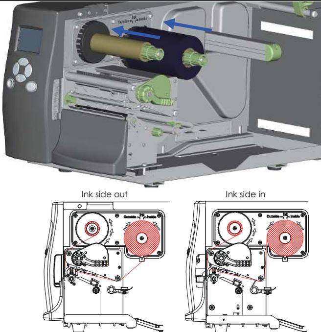
5. Pass the ribbon under the print head and back up on the other side. Attach it to the empty ribbon core.
