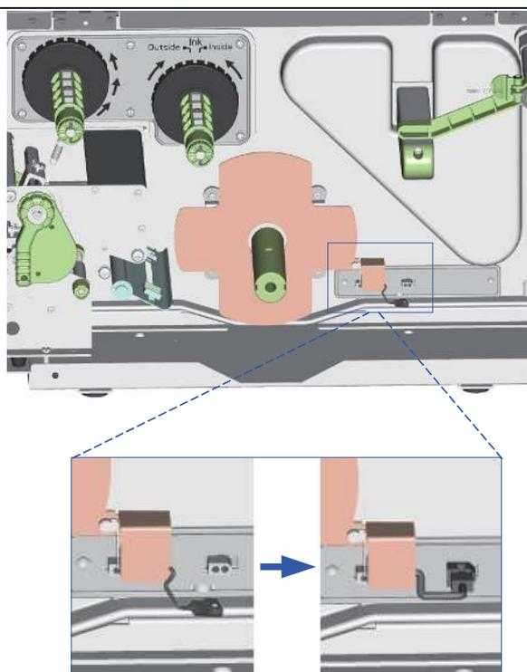
6. Installation of the rewinder module is now complete.
