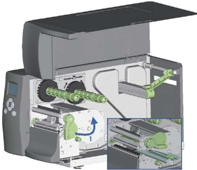
3. Place a new ribbon on the ribbon supply hub. Then place an empty ribbon core on the ribbon rewind hub.
