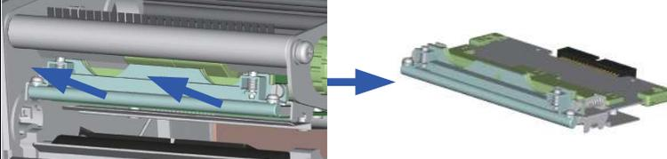
A 3D cutaway illustration showing the print head module being pulled out from the printer. Blue arrows indicate the direction of movement. An inset image shows the module being held.                  |
