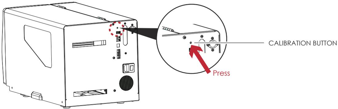
Press C-button for 2 seconds, it will make an auto-sensing to calibrate the label and ribbon's parameters.
