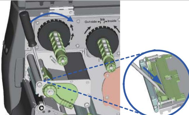
A 3D cutaway illustration showing a screwdriver being used to pry the print head module out of the printer. A circular inset shows a close-up of the screwdriver tip being used to lift the module.     |
