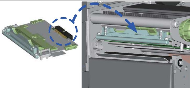
A 3D cutaway illustration showing the print head module being inserted into the printer. Blue arrows indicate the direction of movement. An inset image shows the module being pushed into the printer. |
